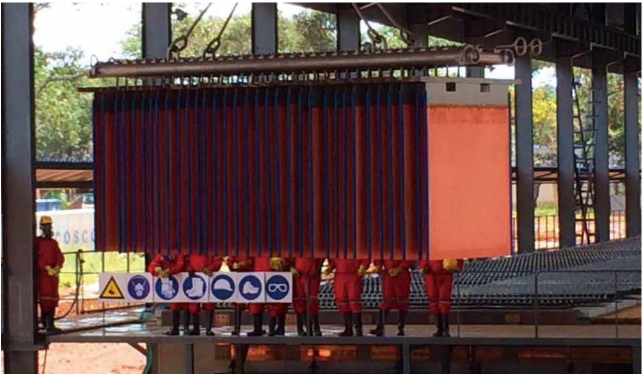
Workers of Mabende Project hoisting copper cathode products (the first batch of products produced in March 2014)
